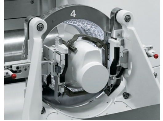
Gamma knife treatment uses focused beams of radiation to treat brain tumors. The Automatic Patient Positioning System (APS) on the Elekta Leksell Gamma Knife® 4C System makes dynamic Gamma Knife radiosurgery possible. Photos courtesy of Elekta, Atlanta, GA, www.elekta.com .
