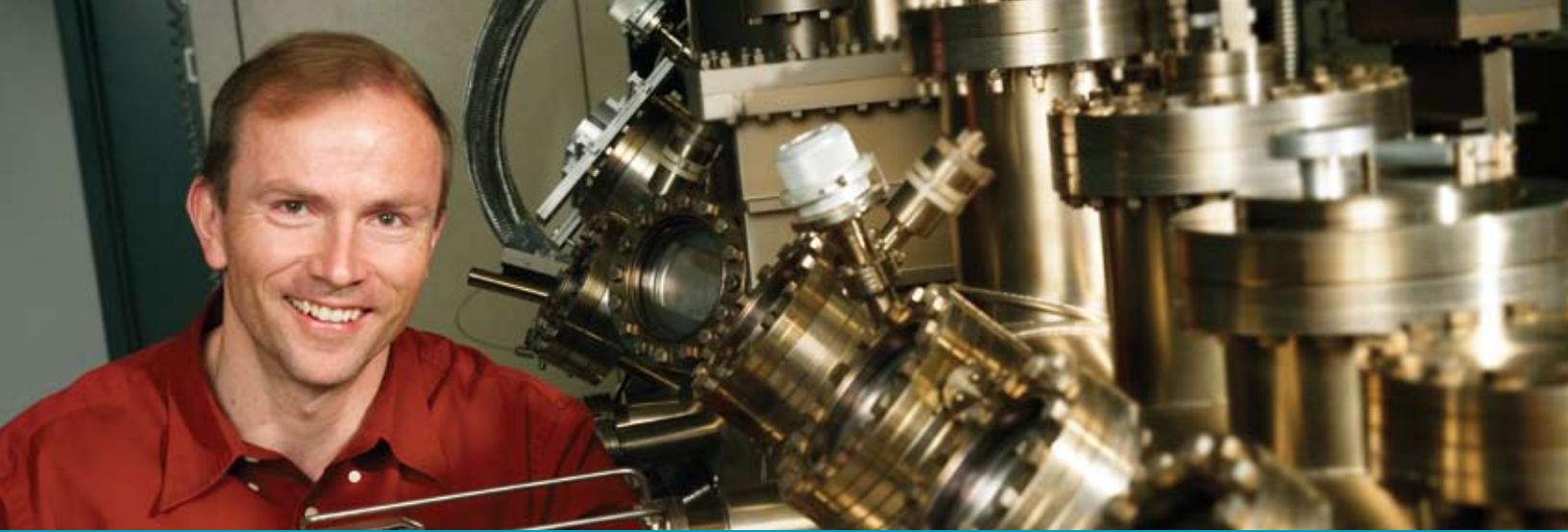
(Above) Zia Laser co-founder and CHTM assistant research professor Andreas Stintz readies the Molecular Beam Epitaxy (MBE) machine for producing quantum dots.
