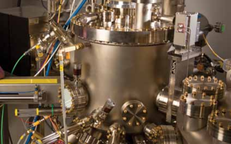
Ganesh Balakrishnan uses the molecular beam epitaxy machine to create novel wafers that could be used as solar cells.
