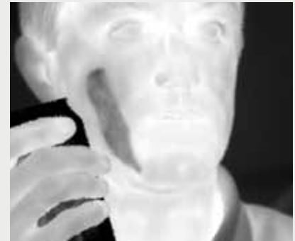
Infrared image taken with a superlattice camera fabricated at UNM capable of measuring temperature differences less than 25 mK. The thermal imprint of a coke can is clearly visible.
